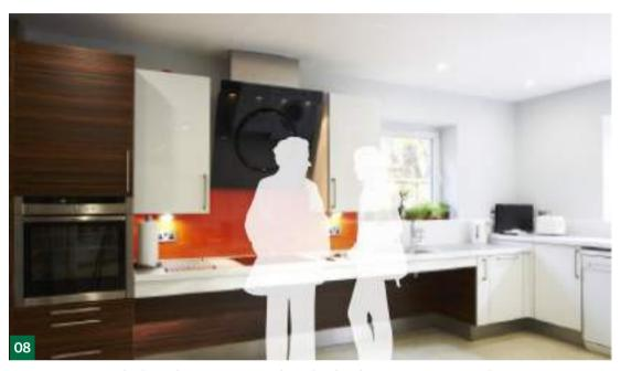
An open space below the counter makes the kitchen easy to use. The counter is lower than standard to suit particular needs.
