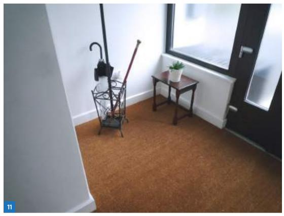
A recessed fixed mat is supplied in the entrance lobby. Good colour differentiation between walls, floor and doors. Space is provided for storage of buggies, wheelchairs or scooters, with a power point for charging.
